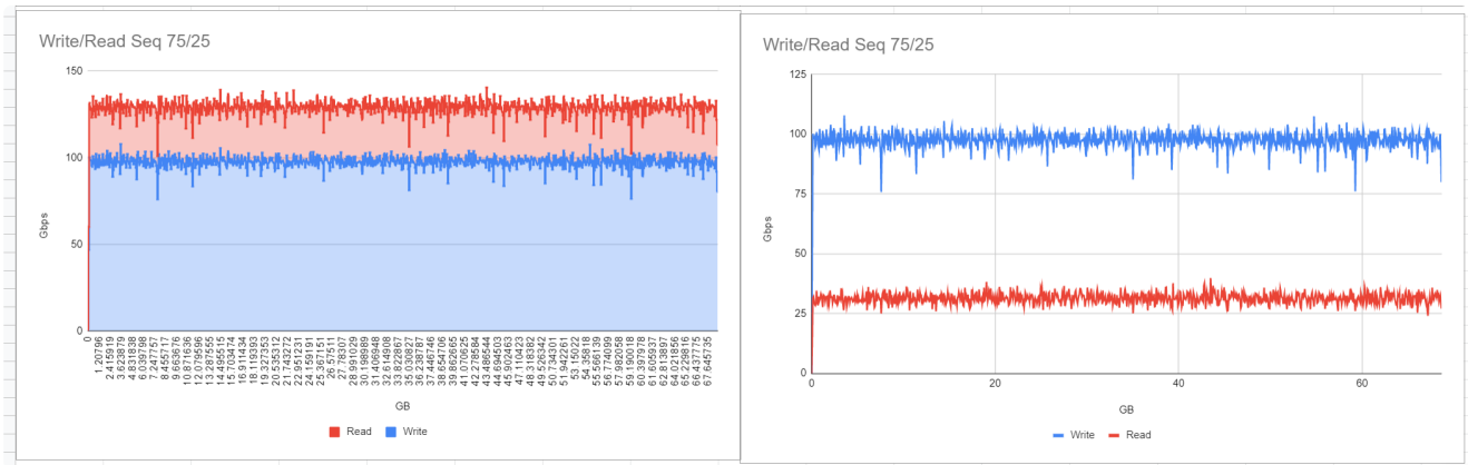
Sustained 100Gbps Capture + 26Gbps sustained Analyze raw IO Throughput
